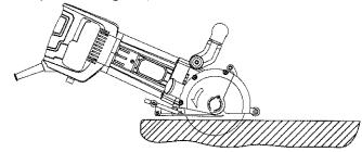
During the slotting make sure the front shield lower to the floor and the back handle to avoid dust splashing.
