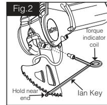
Select the correct blades for the cutting task and mount each with their cap screws. Verify that the surfaces of the blade mounts, conrod thread and screws are clean and free of grit or lubricant before fitting. Ensure the guard can be closed before fixing the blades to the conrod (See Fig.2).
