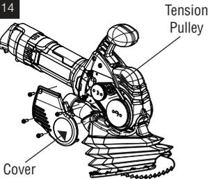
During belt tensioning or replacement a visual inspection of the pulleys should be completed, as they will wear due to excessive belt slip. Replacement may be required if the V profile grooves on the pulleys appear worn or damaged. To replace either pulley contact your ARBORTECH authorised service centre.
