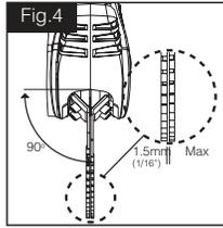
If the gap between the blades is too large, remove and gently bend inward to adjust the gap.
